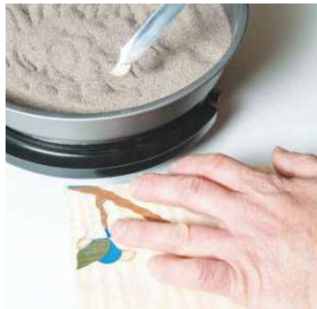
▲ Pic.5 To add depth to the picture, sand shading can be used. Carefully dip the edges in the hot sand, one at a time
